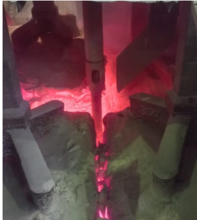
Figure 2. Breaker chisel submerged into liquid bath when in operation.
